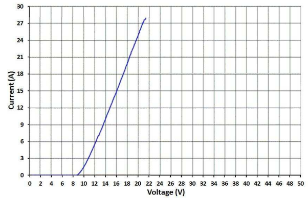
Figure 2. IEC 61000-4-2 Clamp Voltage -8-kV Contact ESD
